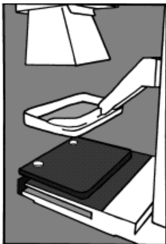
Fig. 2.3 Alignment of X-ray field/image receptor measurement
